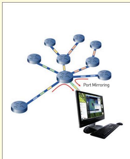
Network flow capture system
