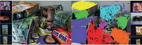
Fig. 2 Deformable feature matching and object detection
